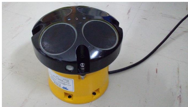
Figure 6 TELEDYNE RDI Workhorse monitor
