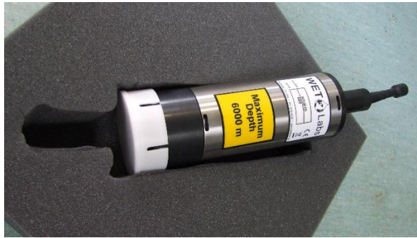
Figure 5 WETlabs ECO NTUrtd
