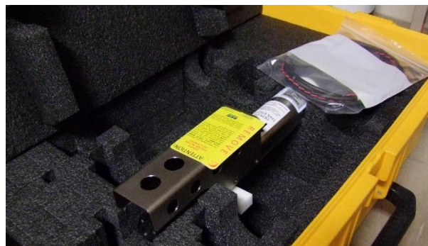
Figure 2 CTD SEABIRD SBE37-SIP-P7000-RS232
