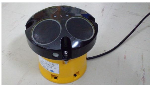
Figure 6 TELEDYNE RDI Workhorse monitor
