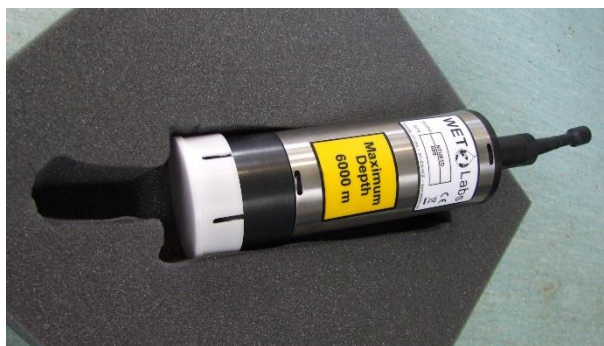
Figure 5 WETlabs ECO NTurtd
